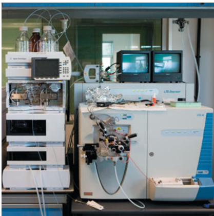
▲ A typical high-performance liquid chromatography (HPLC) system in a research lab (left). The large instrument on the right is a mass spectrometer (Istituto di Ricerche Farmacologiche, Milan, Italy)
