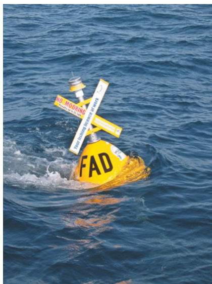
▲ These yellow FADs are not flavins but Fish Aggregating Devices. They are buoys tethered to the sea floor in order to attract fish. This one has been deployed by the government of New South Wales off the east coast of Australia. The strong ocean current is threatening to carry it off.
